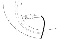
3. Put the air nozzle firmly at the valve nozzle
