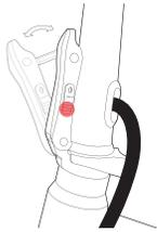
1. Push the handle switch upward and open the handle outwards
